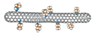
The synthesis and characterization of sidewall amino-functionalized single-walled carbon nanotube derivatives (nPrNH)<sub>n</sub>-SWNTs is reported. The nucle-ophilic addition of in situ generated lithium n-propylamide to the sidewall of
